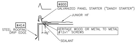
(1.2) GABLE END DETAIL (HIDDEN FASTENERS) (first and last panel)
