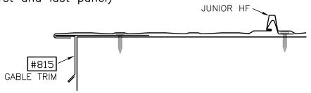
GABLE END DETAIL (EXPOSED FASTENERS) (first and last panel)
