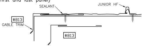
(1.3) GABLE END DETAIL (HIDDEN FASTENERS) (first and last panel)
